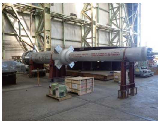
A converter for a green ammonia demonstration plant; Fukushima Prefecture
