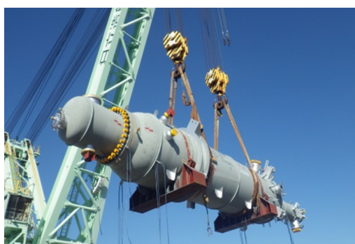
Pressure vessel for fertilizer plants (length 25m, weight 250t)
