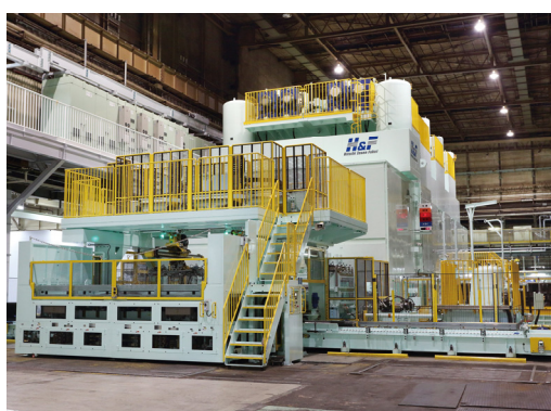
Press machines for automotive industry (servo press line)
