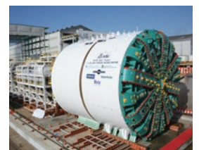
Shield tunneling machine
