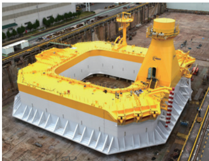
Barge-type floating body of the next-generation floating offshore wind power generation system
