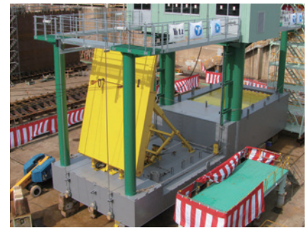
Seabed-mounted flap-gate type seawall (demonstration machine)
