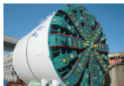
● Shield tunneling machines
