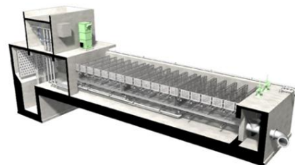
Large-scale fiber filtration system
