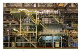
(※) Marine SCR(Selective Catalytic Reduction) system: device that removes NOx emitted from Marine Diesel Engine through a catalyst Business Performance of Marine Diesel Engine (Billion Yen)
