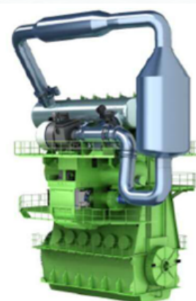
Marine diesel engine equipped with a high-pressure SCR system
