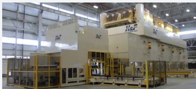
Hybrid servo tandem press machinery production line for automobiles
