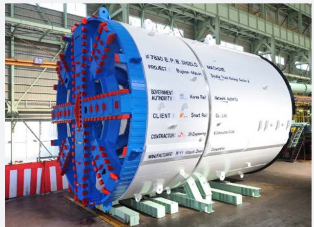
Earth pressure balance shield tunneling machine for construction of the Bujeon-Masan subway in South Korea
