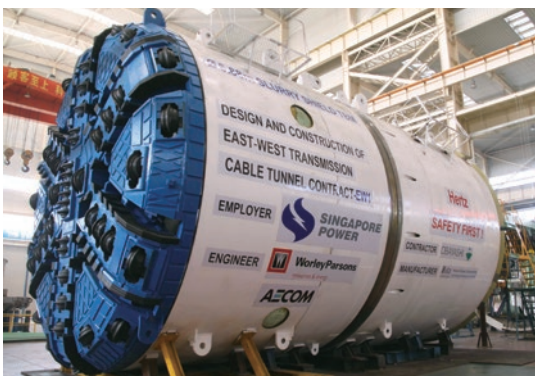
▲ Shield tunneling machine for Singapore
