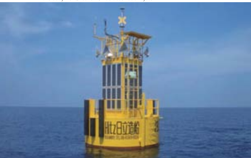
▼ GPS buoy wave/Tsunami/Tide observation system
