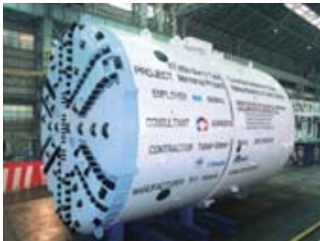
Shield tunneling machine for the Bosphorus
