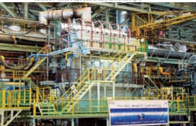
▼ Wärtsilä 6RT-flex 50-B type electronically controlled engine
