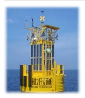
Tsunami of Great East Japan Earthquake is monitored by our GPS Wave Meters.
