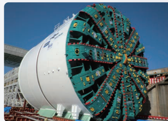
17.45m diameter earth pressure balance Shield Tunneling Machine for the city of Seattle, USA.
