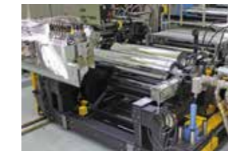
高機能フィルム押出成形テスト機 Highly functional film extruding and forming test machine
